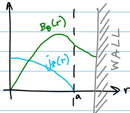
$$\rightarrow \text{screw pinch: } \underline{j} \neq \underline{B} \text{ both helical}$$
