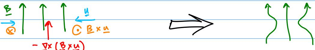
Note 1: Frozen-in flux is NOT always the same as frozen-in magnetic field lines. An ideal MHD plasma can still  $\underline{E} \times \underline{B}$  drift across magnetic field lines so long as the magnetic flux through every volume element is still preserved.
