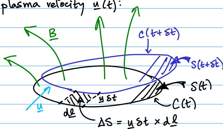
$$\frac{D\phi}{Dt} = \lim_{\delta t \rightarrow 0} \left[ \frac{\iint_{S(t+\delta t)} \underline{B}(x, t+\delta t) \cdot d\underline{s} - \iint_{S(t)} \underline{B}(x, t) \cdot d\underline{s}}{\delta t} \right]$$
