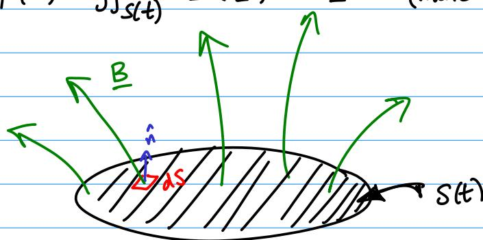
change in magnetic flux through surface  $S(t)$  bounded by contour  $C(t)$  moving with plasma velocity  $\underline{u}(t)$ :
